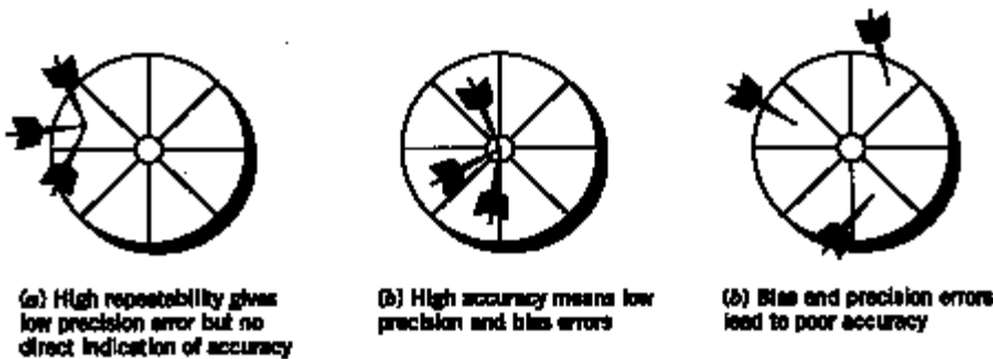
Figure Throws of a dart: illustration of precision and bias errors and accuracy.
